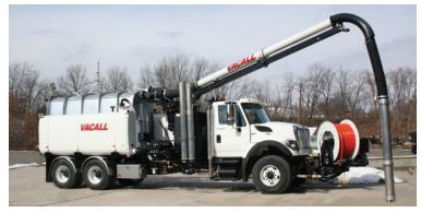
Telescoping boom puts vacuum power where you need it The AllJetVac boom, with the standard 8-foot 6-inch telescopic boom, allows you to place the vacuum power where you need it. The boom's rugged design, lift capacity and rotation will have you spending less time handling the tough jobs and repositioning the unit.
